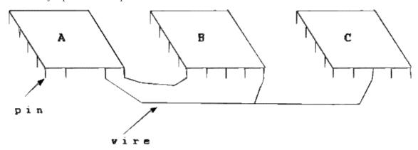
Given a set of pins and a set of wires your task is to determine the number of nets defined within the circuit. The figure below illustrates the circuit with three nets described in the sample input section.
