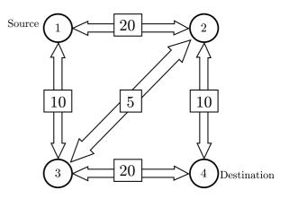
In our example, the bandwidth between node 1 and node 4 is 25, which might be thought of as the sum of the bandwidths 10 along the path 1-2-4, 10 along the path 1-3-4, and 5 along the path 1-2-3-4. No other combination of paths between nodes 1 and 4 provides a larger bandwidth.
