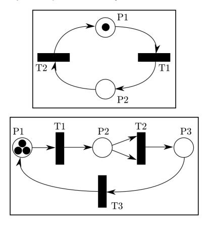
In the first Petri net above, there are two places (P1 and P2) and two transitions (T1 and T2). P1 initially has one token; P2 has none. P1 is an input place for transition T1, and P2 is an output place for T1. In the second example there are three places and three transitions, with three tokens in P1. T2 has two input places, both of which are P2.
