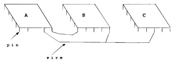
Given a set of pins and a set of wires your task is to determine the number of nets defined within the circuit. The figure below illustrates the circuit with three nets described in the sample input section.
