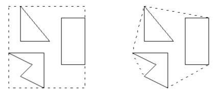
Determining the convex hull of a set of objects is a fundamental problem in both computer graphics and computational geometry. The object of this problem is to write a program that will report the convex hull of a set of simple polygons. An input file will define several such sets of polygons for which convex hulls should be reported in the output file.
