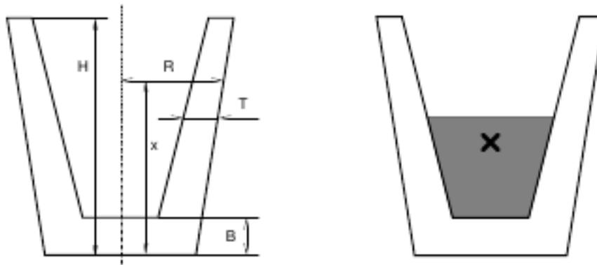
The left figure shows a typical cup considered in this problem. It can be fully described by its height ( $H$ ), thickness of the bottom ( $B$ ), and two functions  $R$  and  $T$ . Both of these functions take a current height as their argument and they give the outer radius ( $R$ ) and glass thickness ( $T$ ) in the appropriate height. Please note that the thickness is always measured strictly horizontally and may therefore not reflect the “real thickness” of the glass in its usual meaning.
