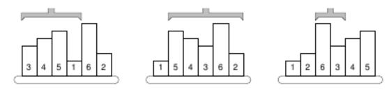
The picture shows a simple example of 6 samples. The smallest one is on the 4th position, therefore, the robot arm reverses the first 4 samples. The second smallest sample is the last one, so the next robot operation will reverse the order of five samples on positions 2-6. The third step will be to reverse the samples 3-4, etc.
