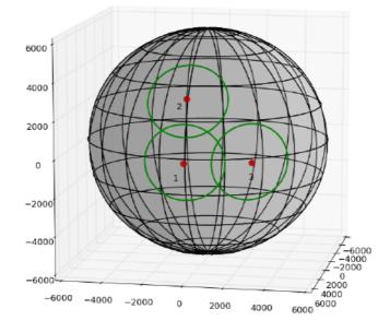
Things are further complicated by the fact that planes have limited fuel supply, and to go longer distances they may need to make a stopover at intermediate airports. Thus, depending on the fuel capacity, a plane going from airport 2 to airport 3 in the figure might have to stop over at airport 1 (or the fuel capacity might be too low even to go to airport 1, in which case the trip would be impossible to make).
