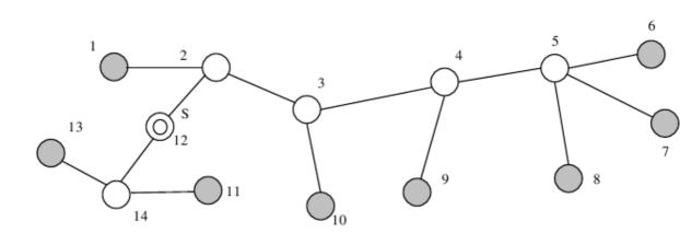
In the above tree, the set of clients is {1, 6, 7, 8, 9, 10, 11, 13}, the set of servers is {2, 3, 4, 5, 12, 14}, and the original VOD server is located at node 12.
