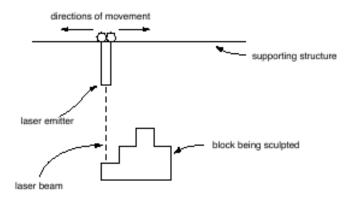
The image above shows a diagram of an equipment to sculpt, with a laser, a block of some solid material. In the figure we can see a laser emitter that moves horizontally to the right and left with a constant speed. When the emitter is turned on when moving, a layer a specific width is removed from the block, being vaporized by the laser.
