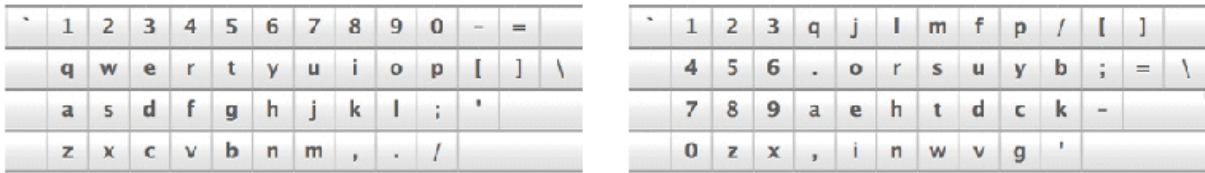
The QWERTY and right-handed Dvorak keyboard layouts arranged on perfect grids.
