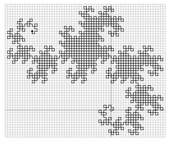
The robot is placed at the origin (the small circle) and face east originally. It ends up at the coordinates (-32,32) (the small spot) after 2048 seconds. The path of the robot is known as a dragon curve, a pretty well-known pattern of fractal.
