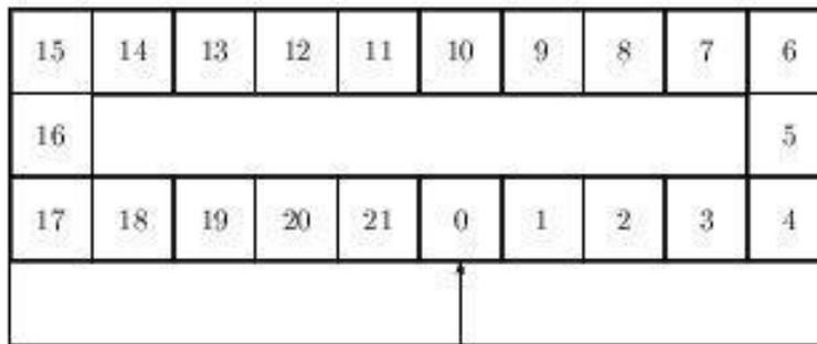
We first read 'D 1' and the program looks for a zone with three hooks free in a row. Since the rail is empty, we select hooks 0, 1, 2 and we store the cloth on hook 1 (hooks 0 and 2 are separators and remain empty). The rail moves and stops when 2 is in front of the mark. So the position is exactly
