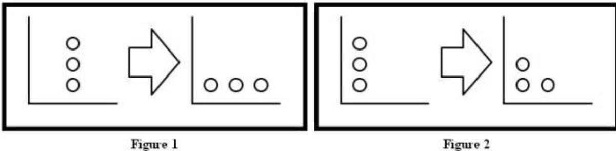
If only one side of the tower is free, for instance if the column is against a wall of the box, then only one ball falls to the free side, and the other one stays on the stack, as shown in Figure 2.
