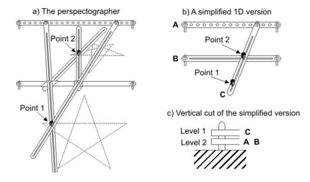
The perspectographer is made of pieces of wood. Some of them are fixed and some others can move along a plane. Besides, some pieces can overlap, so they have to be placed in different levels (i.e., different height). We want to build this machine. How many different levels will we need?
