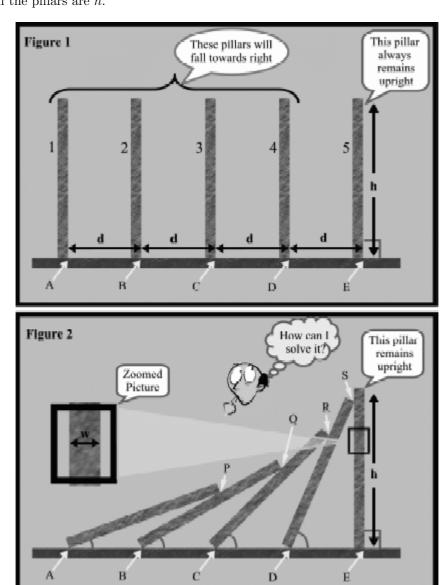
Note that Figure 1, Figure 2 and the Figure below are described as 2-D pictures, which is quite OK for this problem. You must also assume that all the pillars are rectangular and no sliding or lifting occurs when the pillars fall down. Your job is to find out the angles SDE, RCD, QBC, PAB in Figure 2 or other such angles in similar scenario.
