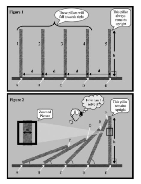
Note that Figure 1, Figure 2 and the Figure below are described as 2-D pictures, which is quite OK for this problem. You must also assume that all the pillars are rectangular and no sliding or lifting occurs when the pillars fall down. Your job is to find out the angles SDE, RCD, QBC, PAB in Figure 2 or other such angles in similar scenario.
