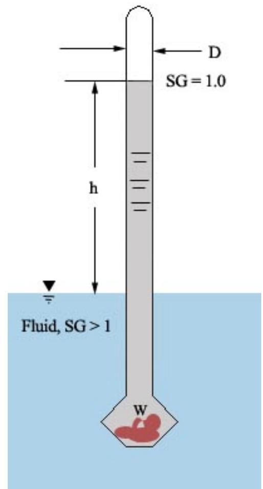
Figure 1 : A Hydrometer
