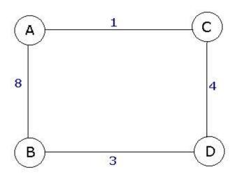
In the above graph road AC is used for route AC,AD,AB. Road AB is used for AB route only. Road BD is used for route BD,BC,BA. Road CD is used for route AD,AB,BC,CD. Thus road CD is maximum used.
