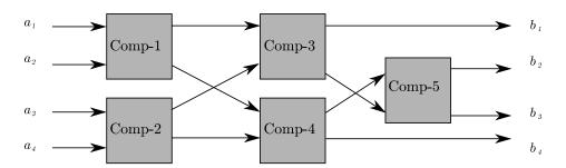
In operation, the network's inputs are applied and the comparators perform their functions. Of course a comparator cannot operate until both of its inputs are available. Assuming a comparator requires one unit of time to operate, this sample network will require three units of time to produce its outputs. Comp-1 and Comp-2 operate in parallel, as do Comp-3 and Comp-4. Comp-5 cannot operate until Comp-3 and Comp-4 have comp leted their work.
