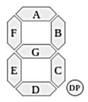
Figure 1: Segments used for SSD representation. Here, DP represents decimal place which is not necessary in the context of this problem.
