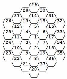
First level is the center and it contains only cell 1. The number of cells in subsequent levels is 6,12,18,....  $2^{nd}$  level contains cells from 2 to 7,  $3^{rd}$  level contains cells from 8-19,  $4^{th}$  level contains cells from 20-37,... In each of the first the lowest cell is numbered. Then the rest of the cells are numbered in clockwise order.
